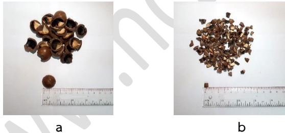
Figure 2 Photograph a) Macadamia nut shells b) Grounded macadamia nut shells (0.5x0.5 cm)
